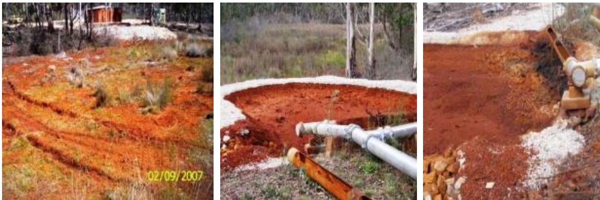
Photos: Invincible Colliery LDP001 discharge into Coxs River – 2/09/2007. EC 1710 \mu\text{S}/\text{cm} , pH 6.5, DO 0%, Anoxic odour
