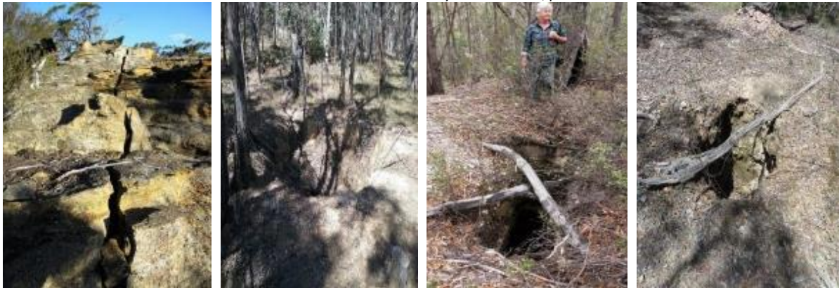
Photos: Invincible Colliery mine subsidence damage to pagodas, sinkholes, and open mineshafts
