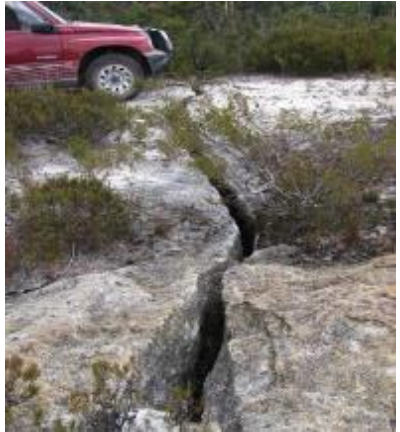
Photos: Cliff fall and subsidence cracks on Newnes Plateau above Cobar Park Colliery bord & pillar workings – March 2009
