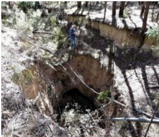
Photos: Invincible Colliery – Creeks disappearing down subsidence cracks into mine void – 19 August 2017
